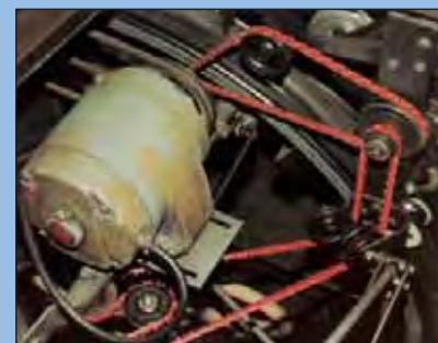
**Solution** Making to length and installing quick connect PowerTwist Plus V-Belts can be accomplished with nothing more than a flick of the wrist.
