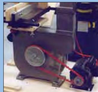
**Solution** Fitting PowerTwist Plus HPC V-Belts damped transmitted vibrations and reduced system noise significantly. All belt-driven woodworking equipment will benefit from fitting the red belt — perfect cuts and finishes every time!
