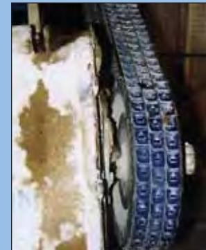
**Solution** Fitting high performance SuperTLink provided greater resistance to the harsh operating conditions. Belt life was increased five times with the TLink belt design absorbing vibratory stresses.
